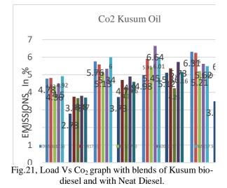
The variations of carbon dioxide emission for various blends at varying loads are shown in figure 21. The carbon dioxide emissions for the blends are higher than diesel for all loads and blends and decreases with compression ratio. Carbon dioxide is formed on complete combustion of the fuel in oxygen. As the calorific value of the fuel is low, more fuel needs to be burnt to get equivalent power output. So combustion of more carbon compounds leads to higher carbon dioxide emissions.
