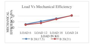
Fig.8, Load Vs Mechanical Efficiency graph with B20 blend of kusum bio-diesel at various loads.
