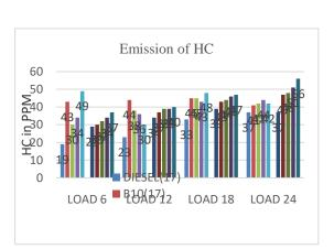
Fig.22, Load Vs HC graph with blends of Kusum biodiesel and with Neat Diesel.
