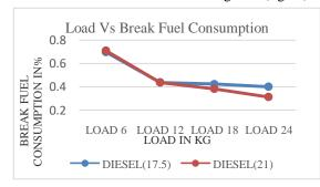
Fig.15, Load Vs Break Fuel Consumption graph with Neat Diesel at various loads.
