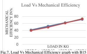
Fig.7, Load Vs Mechanical Efficiency graph with B15 blend of kusum bio-diesel at various loads.
