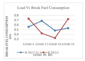
Fig.18, Load Vs Break Fuel Consumption graph with B20 blends of kusum bio-diesel at various loads
