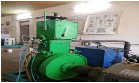
Fig.1, Computerized VCR engine test rig
