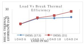
Fig.10, Load Vs Break Thermal Efficiency graph with Neat Diesel at various loads.
