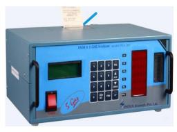
Fig.2, Indus pea 205 Exhaust Gas Analyzer
